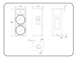
K25A is the extremmly high power speaker with extended low-end output. The special 2,5-way design allows to use both 15" transducers for low-shelf reproduction, with only the upper one used for mid range, providing clarity and smooth vertical coverage pattern. State-of-the-art amplification from Powersoft adds to ease and convenience of use.
